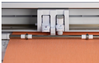
Rotary Blade for cutting cotton fabrics, leather, felt and more ( Optional item )
